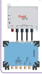
If you have a Quad GTU, the engineer will need to connect a DCSS switch to it, to allow you to receive Sky Q services.
